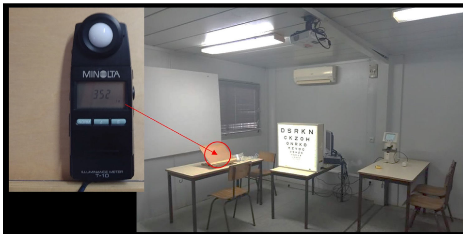
Fig. 1 The right image shows the experimental setup of the room used for obtaining measurements using the MNREAD chart. The natural light was avoided by pulling down the blinds, the chair where participants sat to measure acuity is not in the picture. The table, chair and reading tray used for the MNREAD test is visible highlighted by the circle. In the magnified left image highlighted by the arrow and a circle shows the luxmeter with an illuminance (Il) reading of 352 lx that can be converted to luminance (L) using the formula: L = Il \times \text{reflectance}/\pi . Assuming a reflectance of 95% for the white background of the MNREAD test, the luminance in the test would be 106 \text{ cd/m}^2 . The focimeter that was used to measure the habitual spectacle correction is also visible in the picture.
