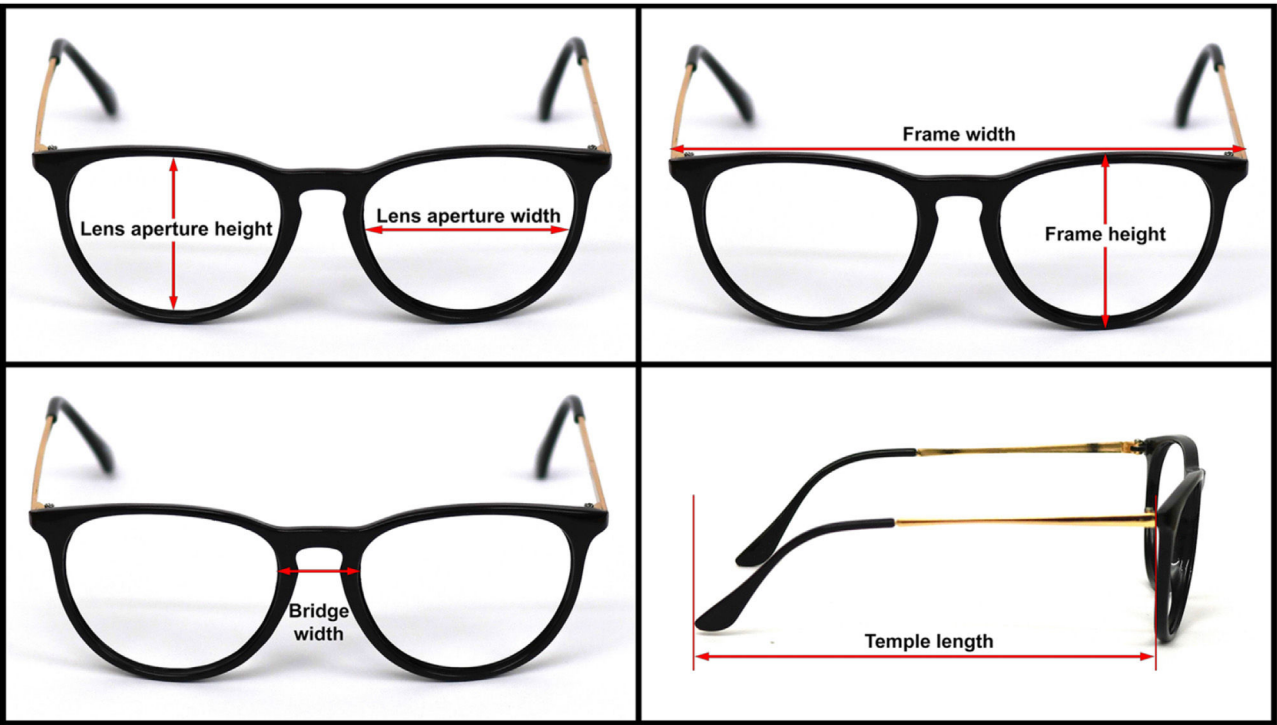
Fig. 2. Spectacle frame measurements.
