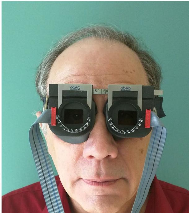
**Figure 2** An image of the OBER2 recording system (Permobil/IOTA Eye Trace) with the second author pictured as the subject.
