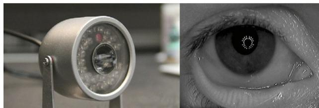
**Figure 2** An infrared security camera modified for meibography (left). A ring of infrared LEDs illuminate the eye, and the central camera unit captures infrared video to be displayed on a computer screen (not shown). The inferior lid is everted to reveal MGs in infrared light. This image was captured by the modified security camera. The ring configuration of the infrared LEDs of the camera can be seen in the reflection of the cornea (right).
